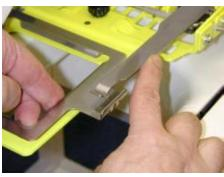
With clamp in the "open" position, slide the upper clamp plate under the spring arms and engage one of the "pivot lugs" in the center slot of the clamp plate. While holding the clamp plate on the lug, flex the other arm toward the middle of the clamp and engage the other side.
