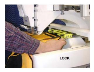
A benefit of loading in the machine is that you can verify that the garment is "lined up"
